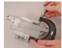
Above: Set S154LZ with 154E in foreground Right: Checking inside measurement of slot with parallel and outside micrometer
