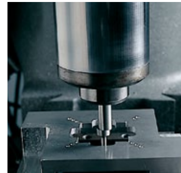
Locating the edge of a part with 827MA
